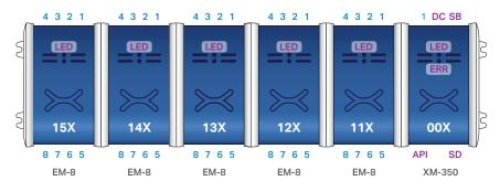
DC. 5VDC Power input (2.5mm DC socket)
